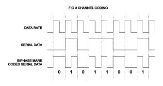
violate this coding format, i.e. they do not have transitions on all of the bit boundaries. If this coding structure is violated elsewhere, the **LM1** indicates a bi-phase error.
